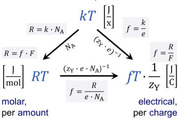
**Table 1.** Motive force quantum defined by SI constants (k,  $N_A$ , and e) and expressed in different formats of the Boltzmann constant k, gas constant R, and electromotive constant f. Values of these quantum effects are shown for the standard temperature of 25 °C ( $T^\circ$  = 298.15 K). The motive force quantum at any temperature T is obtained by multiplication by  $T/T^\circ$ . Multiplication factors for 0 °C and 37 °C are 0.916 and 1.040, respectively;  $\ln(10) \approx 2.3026$ .
